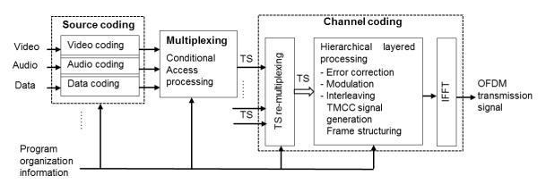
Fig-2 Block Diagram of ISDB-T DTTB transmission System
