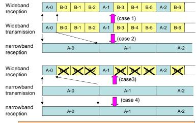
As shown above, output TS rate of narrow band receiver is lower than wideband receiver (in general, 1/8 of wideband receiver)
