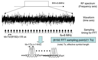
5617 subcarrier(=5.6 MHz) are used for data transmission
