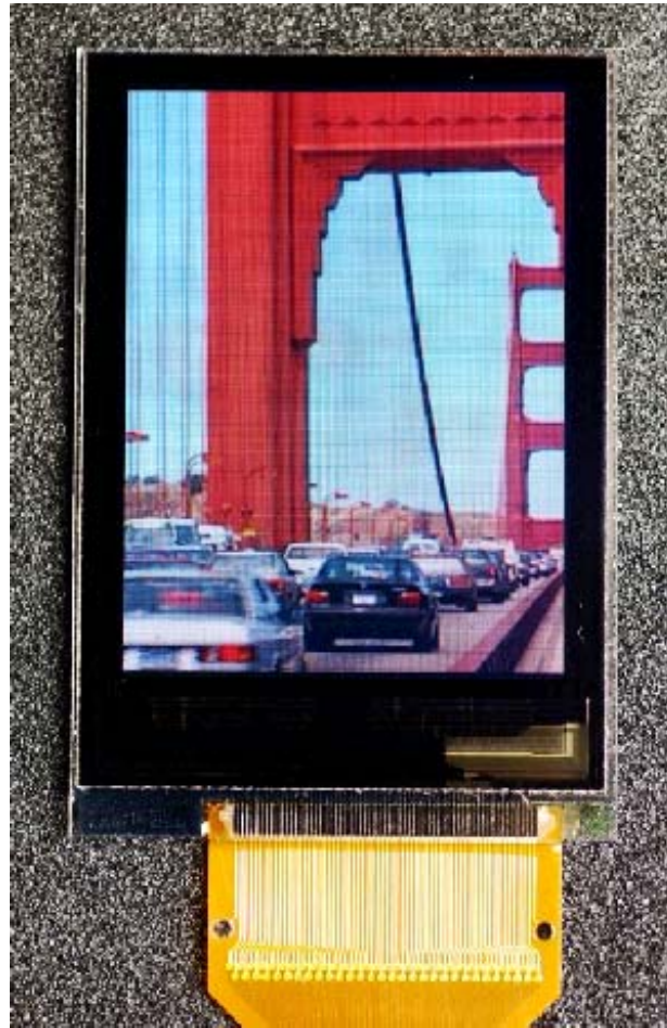
2.4 inch Active Matrix Full Color Film OLED (prototype)
