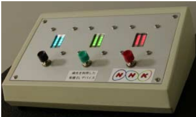
Phosphorescent Polymer-based EL Display
